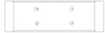
H08 (x1) SUPPORT DE CHEVRON - W4L17530 15/16 po x 3 3/8 po x 10 11/16 po (24x86x272)
