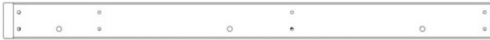
H30 SUPPORT DE CHEVRON - W4L17570 (x1) 15/16 po x 3 3/8 po x 46 3/8 po (24x86x1177)
